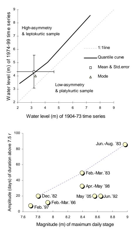
**Fig. 3:** Above: comparison of 1904-73 and 1974-99 water level records at Corrientes Port. Below: extraordinary floods (1904-99) with the 1982-83 ENSO outlier (dashed lines).
